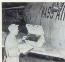
The Type 1429-A Fuel-Gage Tester (TTU-68/E) in operation at an Air National Guard Base.
