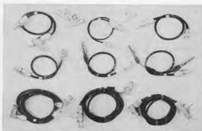
Figure 2. Connectors to fit many types of fuel gages are furnished with the tester.
