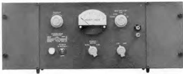
Figure 5. Panel extensions are furnished to adapt the instrument for relay-rack mounting.
