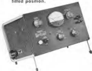
Figure 4. Extendible legs allow instrument to be used in a tilted position.
